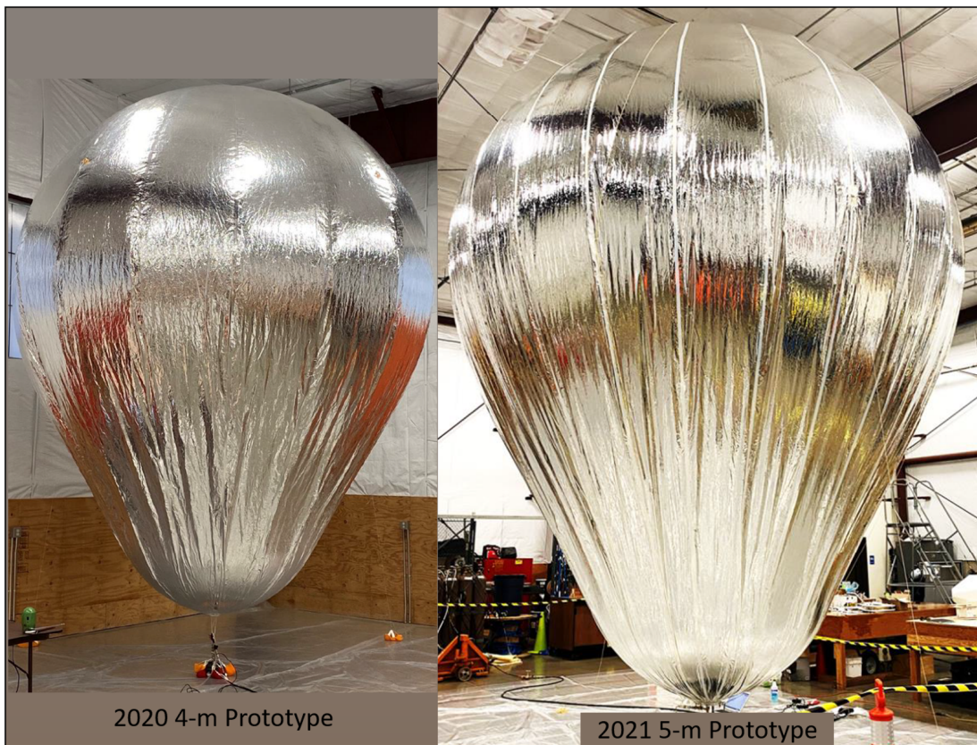
Figure A.10: Two sub-scale prototypes of a Venus variable-altitude aerial platform. Images reproduced with permission from Izraelevitz 2022.
