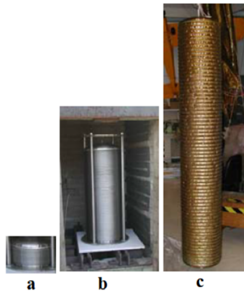
Figure A.18: 0.35-m diameter metal bellows at (a) \Delta P = -84 mB, (b) \Delta P = 114 mB, (c) \Delta P = 630 mB after exposure to +460^{\circ}\text{C} .
