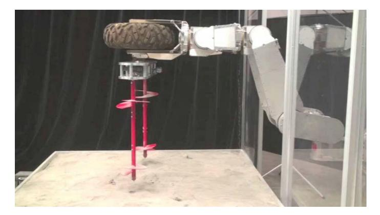
Counter-rotating helical augers have no net torque reaction. Separation between flutes reduces friction without reducing pull-out force compared to continuous flute.
