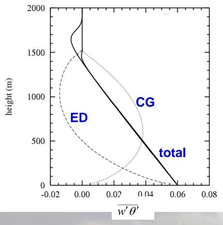
$$\overline{w'\theta'} = -K\frac{\partial\overline{\theta}}{\partial z} + K\gamma$$
