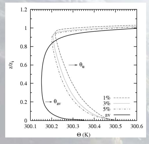
Updraft at height z composed of those grid points that contain the highest p% of the vertical velocities: p=1%,3%,5%:
