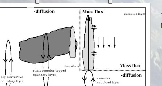
$\left|\frac{\partial \phi}{\partial t} \cong -\frac{\partial}{\partial z} \left(\overline{w' \phi'}\right) + \overline{S}\right|$
