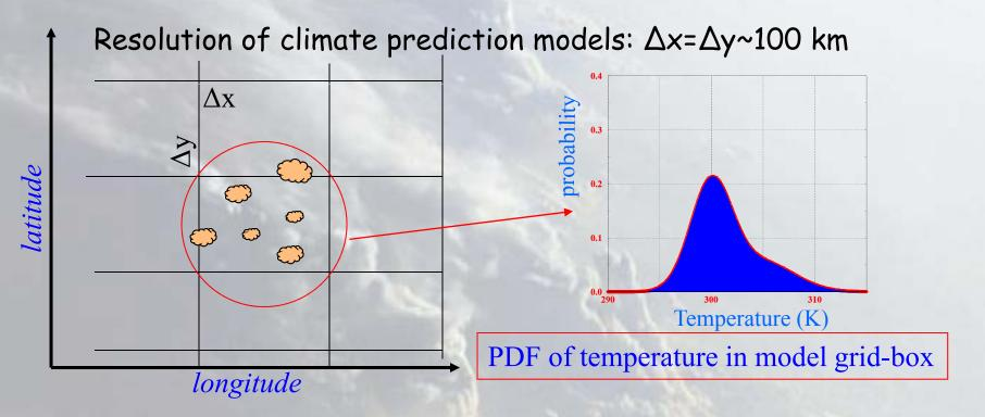
Essence of parameterization problem is the estimation of joint PDFs of climate model variables (u, v, w, T, q) -> e.g. co-variance  $w'\phi'$
