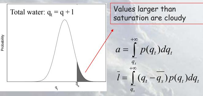
With Gaussian distribution we obtain cloud fraction and liquid water as a function of Q:
