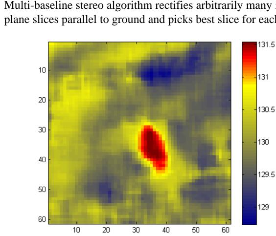
Elevation map for cropped region around car. Area around car ~1.5 m higher than neighboring ground plane. Higher image resolution might address some remaining noise issues.
