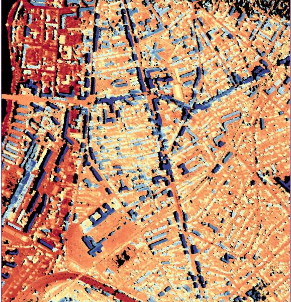
DSM generated with a tri- stereoscopic couple. Toulouse 2012
