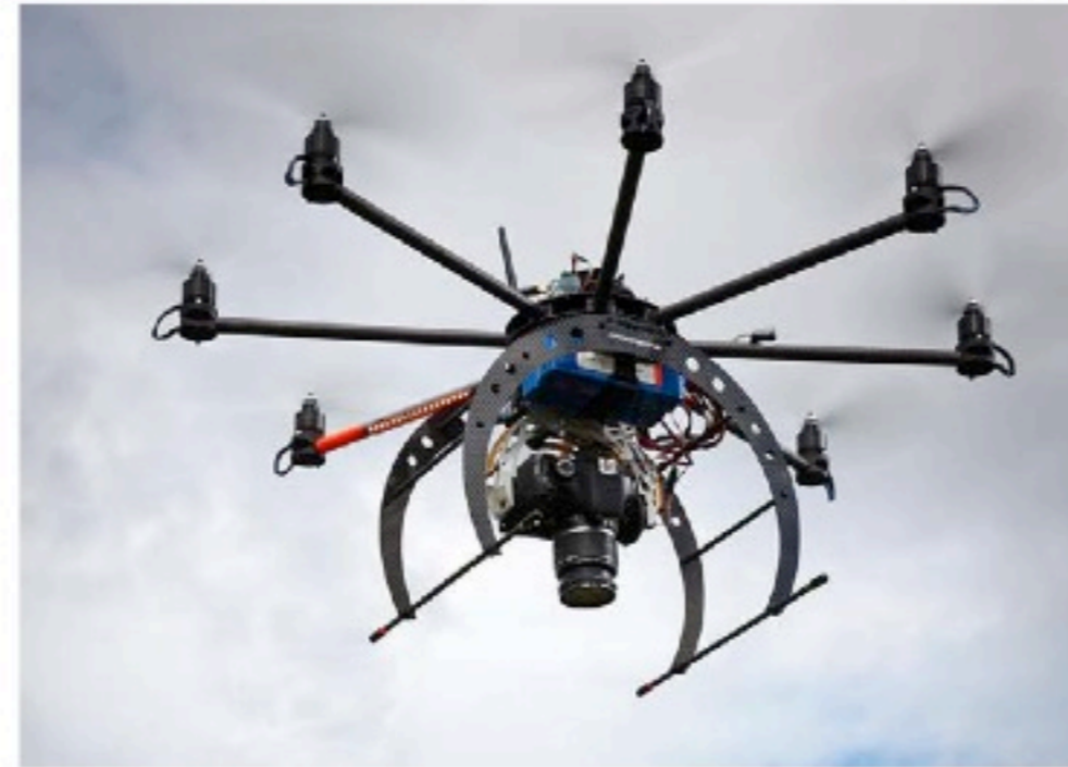
Figure 3. The remote controlled UAV OktoKopter equipped with digital camera and GPS.
