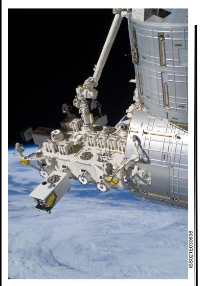
Japanese Experiment Module-Exposed Facility (JEM-EF) attached payload for the International Space Station (ISS)
