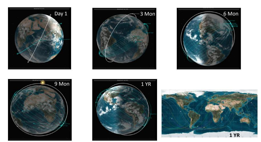
Immediately after launch, all satellites (blue lines) are in the same orbit plane. Due to slightly different precession rates (due mostly to different satellite altitudes), the satellite orbits spread over time such that within a year they are spread equally over the globe.
