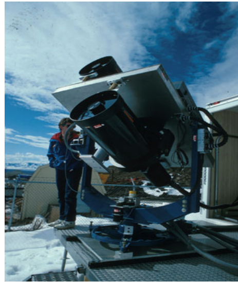
• Polarization Diversity Lidar (PDL) Scanning, 0.532 + 1.06 \mu\text{m} , 10 Hz PRF
