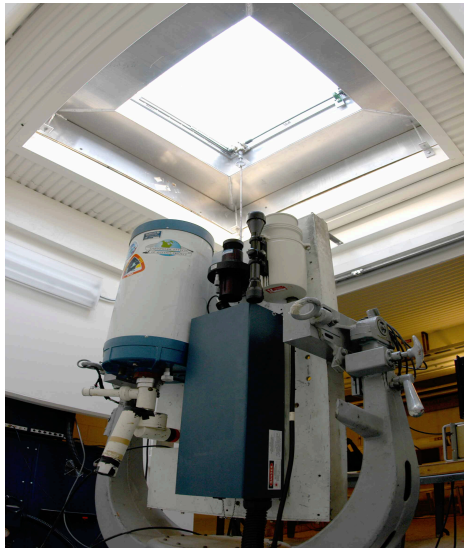
Cloud Polarization Lidar (CPL) 0.694 \mu\text{m} 0.1 Hz PRF
