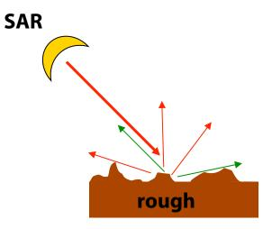
Multiple bounce backscattering on a rough surface randomizes polarization (OC ≅ SC)
