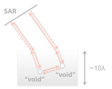
Forward scattering in ice preserves polarization (OC << SC) HIGH CPR (> 1)
