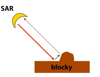
Blocky surfaces may act as corner reflectors, causing double bounce backscatter (OC << SC)
