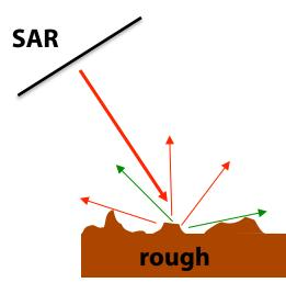
Multiple bounce backscattering on a rough surface randomizes polarization (OC ≅ SC)
