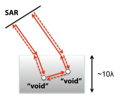
Forward scattering in ice preserves polarization (OC << SC) HIGH CPR (> 1)
