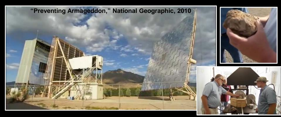
Melosh: Rock samples placed in "solar furnace" designed to simulate heat from nuclear blasts.
