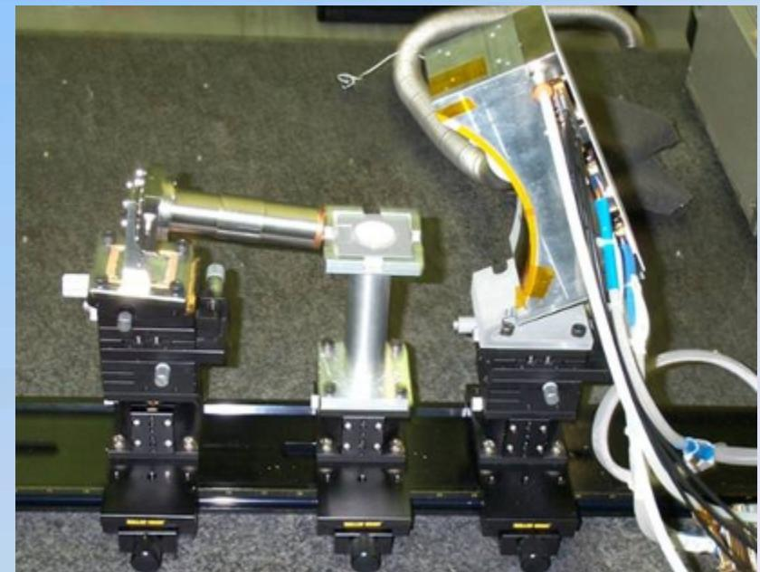
$^{55}\text{Fe}$  self-emitting X-ray source prototype
