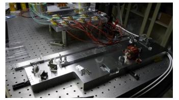
Compact Fiber Laser Demonstrator Facilitates compact, ruggedized high energy, pulsed fiber opto-mechanical assemblies Demonstrated operation at power with only a 2.5% loss (32.5% bus-plug)
