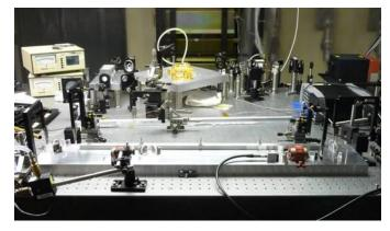
High Efficiency Fiber Amplifier Testbed Validated fiber laser efficiency advantage over conventional solid state laser systems Demonstrated 33.5% bus-plug efficiency to date
