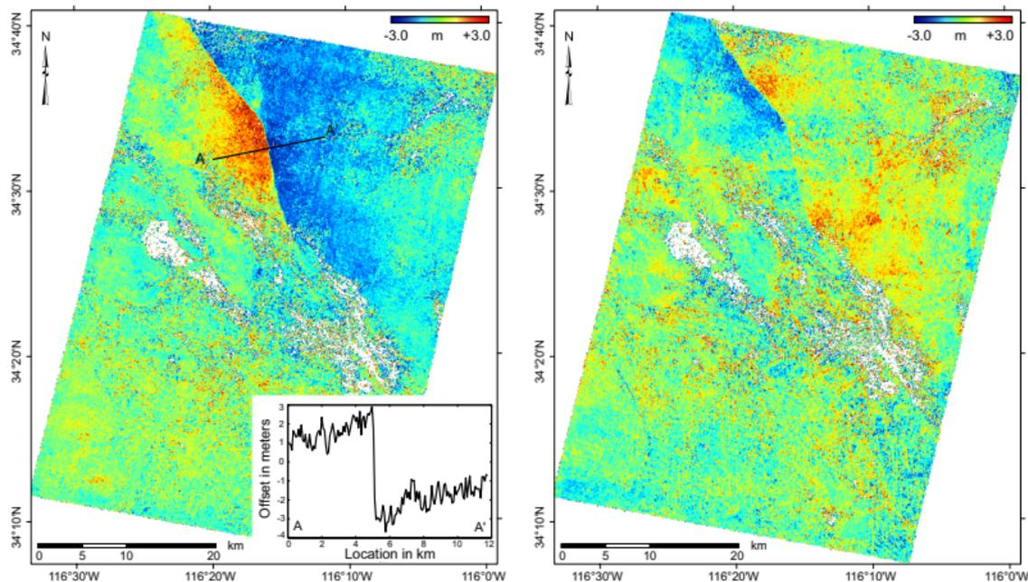
The Hector Mine horizontal coseismic field (NS and EW) once CCD distortions from SPOT4 and SPOT2 have been modeled during orthorectification. **Accuracy better than 1/10 pixel.**
