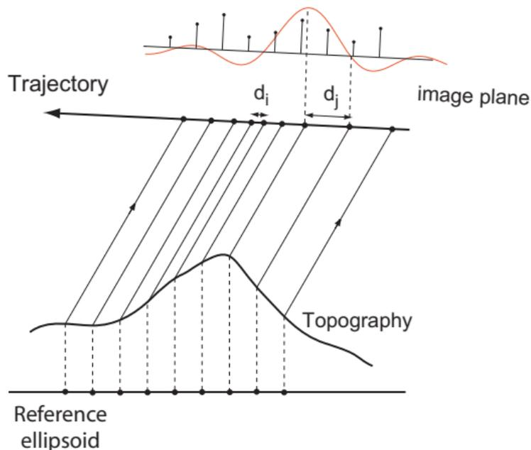
Resampling irregularities depend on the local viewing angle and topography gradient. They increase with image resolution and **can vary by up to a factor of 10** in high resolution images over steep topography.
