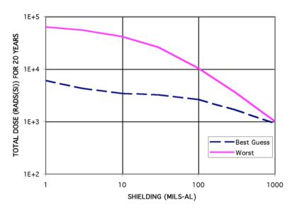
Total Ionizing Dose from Galactic Cosmic Rays as a Function of Aluminum Shielding Thickness Graph\*. Units are Rad(Si) vs Mils(Al)
