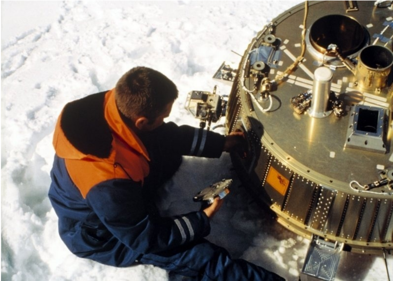
SM2 - Parachute drop test from 40km balloon over northern Sweden, 1995 Successfully demonstrated heat shield separation/parachute sequence. Deviant rotational behavior not noticed at the time.
