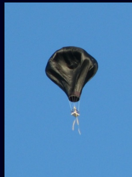
Successful aerial deployment and inflation test on 4.5 m balloon (300-400 meter altitude)
