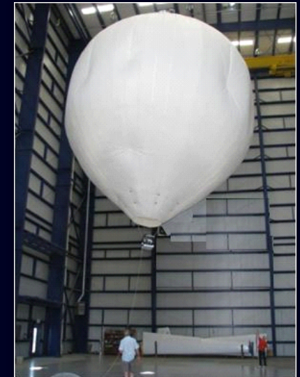
Indoor propane-heated flight of 9 m prototype
