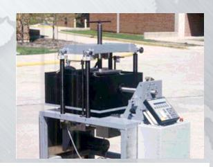
12"x12" Direct Shear Device at UIUC
