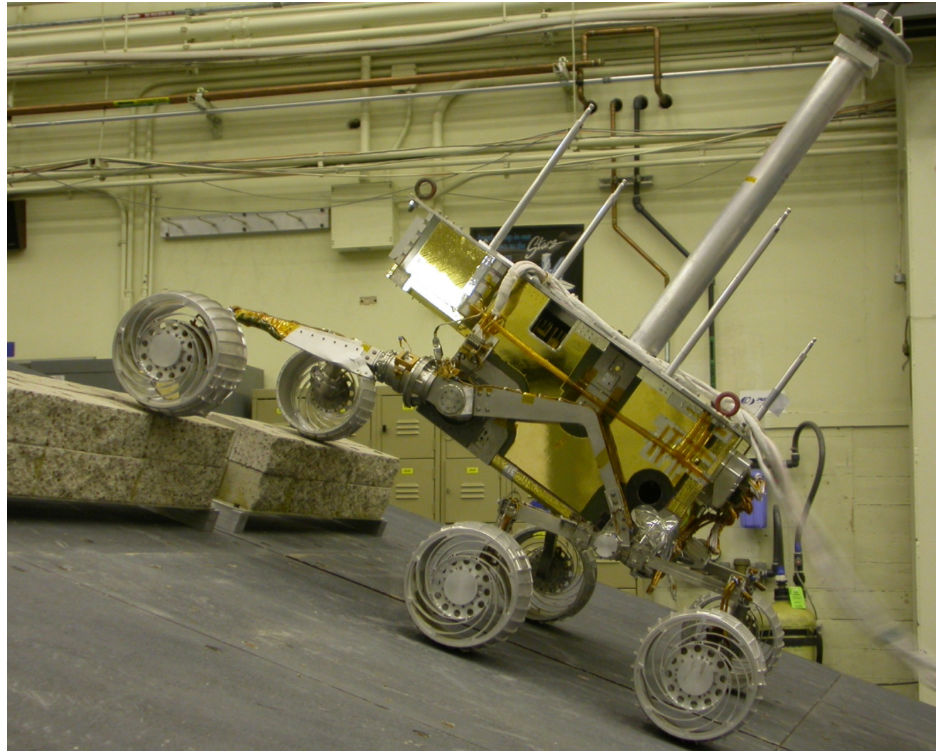
Dynamic Test Model rover driving up a 15 deg slope, climbing a 25 cm obstacle
