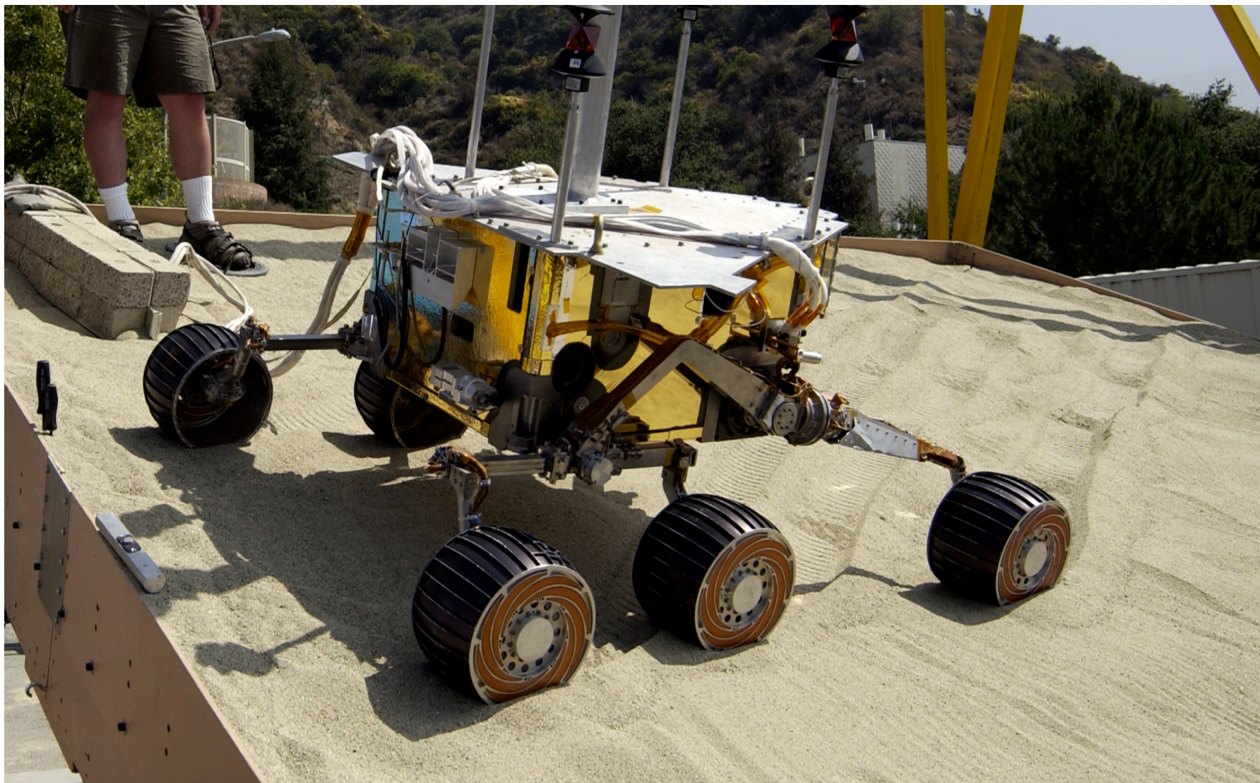
DTM Rover driving cross-slope on the VTT, at a 20 deg slope, and covered with 20 cm of dry, loose quartz sand
