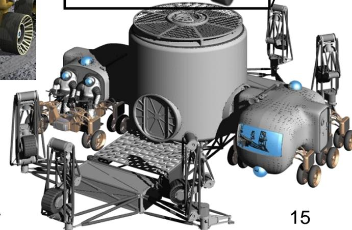
All struts have ball-ends and so can be loaded only in compression or tension.
