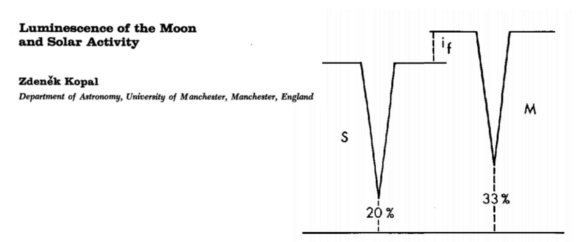
FIGURE 9-2: The line-depth method of detecting luminescence calls for comparing profiles of absorption lines in the spectra A of the sun (left) and moon (right). An increase in the residual intensity in the case of the moon is a measure of the light  $(i_F)$  attributable to lunar luminescence—in this example 16.67 per cent of the total moonlight.
