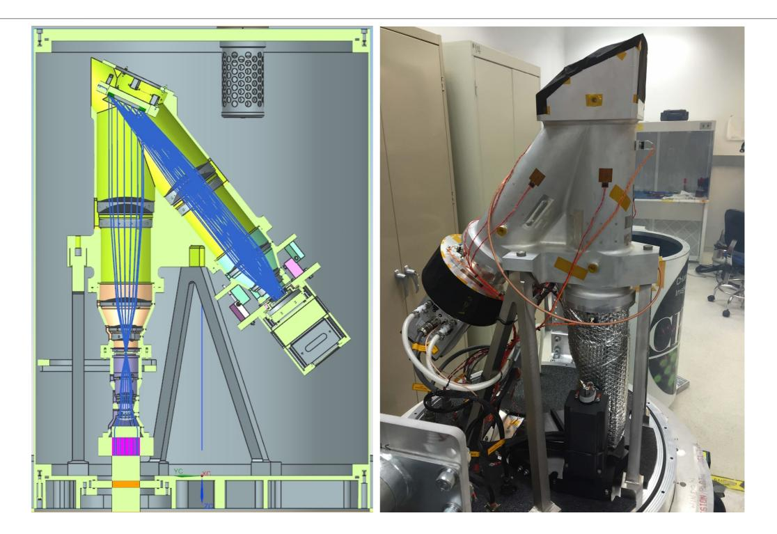
Figure 2: Left: CFIS computer-aided design model, showing the mechanical and optical layout. Right: Picture of CFIS without housing can in the laboratory.
