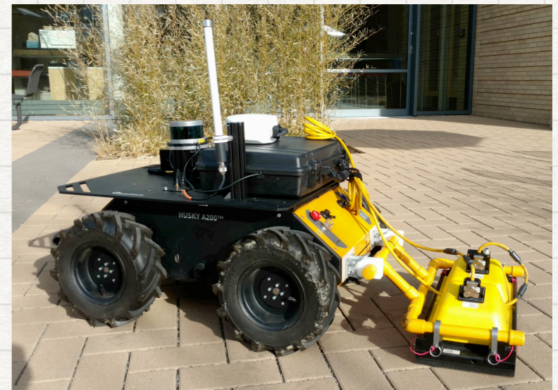
The Colorado School of Mines Geobot . An autonomous survey tool that can be remote controlled or follow a pre-programmed path. Here it is outfitted to perform GPR surveys, but it could be used to transport seismic sources or wireless receivers.
