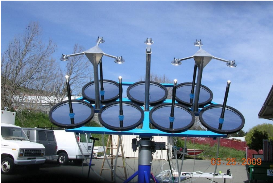
Seven concentrators mounted on the tracking array
