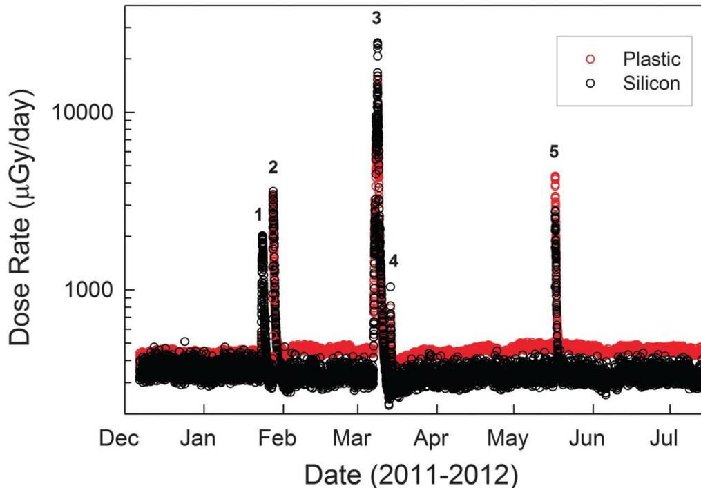
**Figure 2.8:** Dose rates from Curiosity's RAD instrument, in the silicon and plastic detectors, during the cruise phase to Mars. The background level at approximately  $400 \mu\text{Gy d}^{-1}$  is the effect of the ever-constant GCRs, while the impulsive emission near or exceeding  $10,000 \mu\text{Gy d}^{-1}$  represents the effects of passing SEP events. [Figure from *Zeitlin et al. (2013)*]
