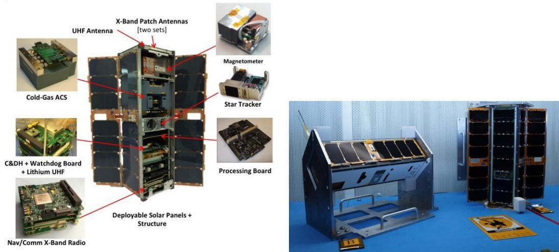
**Figure 4.5:** (Left) Interplanetary NanoSpacecraft Pathfinder In a Relevant Environment (INSPIRE) cubesat design. Intended as pathfinders, the INSPIRE spacecraft will prove the cubesat concept for deep space and could serve as the platform upon which to base a future radio astronomy mission for detecting the magnetospheric emissions from extrasolar planets. (Right) The two INSPIRE spacecraft ready for launch. At the time of this writing, no launch date has been set.
