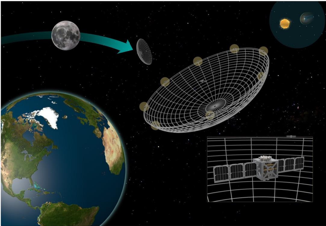
**Figure 4.6:** Artist's illustration of how a large diameter single aperture could be realized in space. In this concept, small spacecraft ("cubesats") would control the shape and steering of the telescope. Moreover, while the focus of this work is on the use of such a telescope for studying extrasolar planets, it might also be able to be used for studies of the highly redshifted neutral hydrogen hyperfine line from the Cosmic "Dark Ages."
