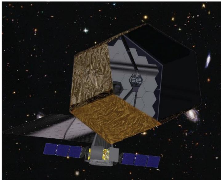
**Figure 4.9:** Artist's impression of one concept for the ATLAST flagship observatory, optimized for observations in the ultraviolet to visible wavelength spectral range. This figure shows a 16-m-diameter aperture after having been deployed. [Credit: STScI.]
