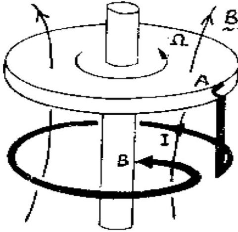
**Figure 2.2:** Mechanical analog to a magnetic dynamo. In the disk dynamo, the electromagnetic force (EMF) created by disk rotation creates a current that produces the field responsible for the EMF.
