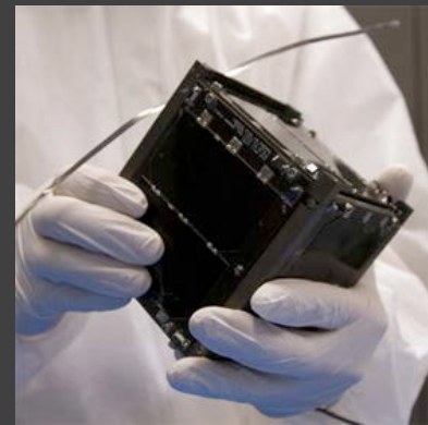
1U CubeSat with dimensions of 10x10x10 cm (Courtesy Cal Poly San Luis Obispo)
