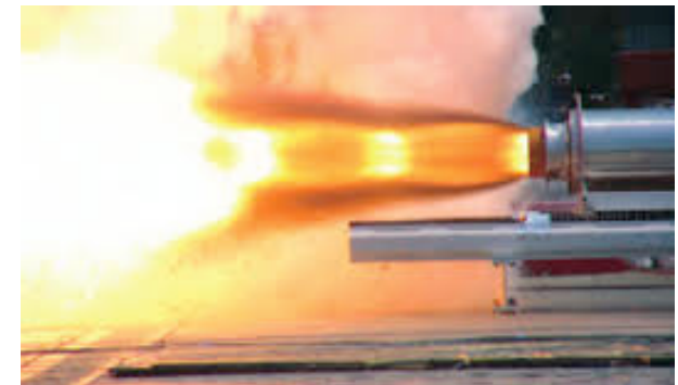
Peregrine Motor Test, NASA Ames, Source: Aerospace America 2011.
