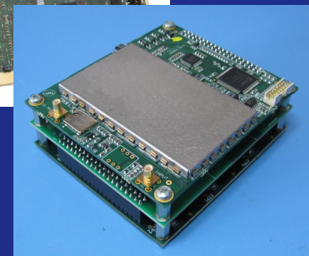
Example CubeSat capable GPS receivers (Novatel and FOTON)
