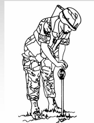
Figure E-3. Using a cone penetrometer in the upright position
