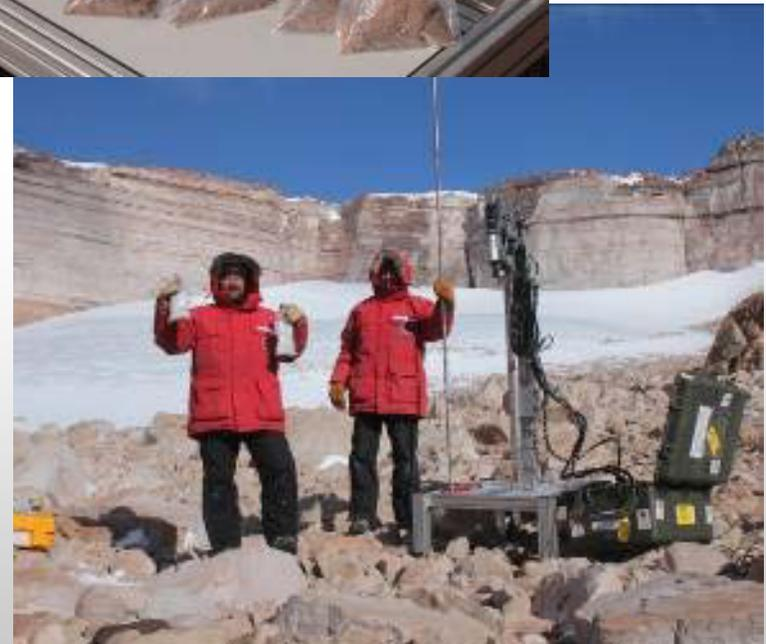
Honeybee Robotics IceBreaker rotary-percussive drill prototype being tested in Antarctica
