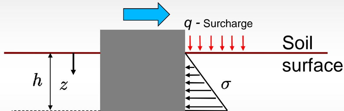
$$\sigma = \gamma z N_{\gamma} + c N_c + q N_q \text{ [Pa]}$$
