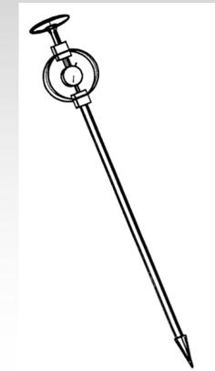
Figure E-2. Cone penetrometer
