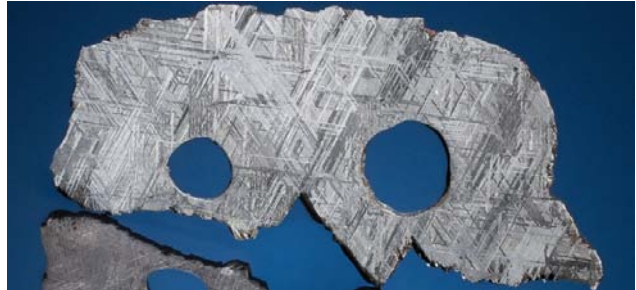
Figure 6: The Widmanstätten pattern, which is found only in meteorites – and hence in asteroids – forms over millions of years of cooling at rates of 100 – 10,000 C/million years, and experiment not reproducible on Earth. Other “meteorite materials” are known.
