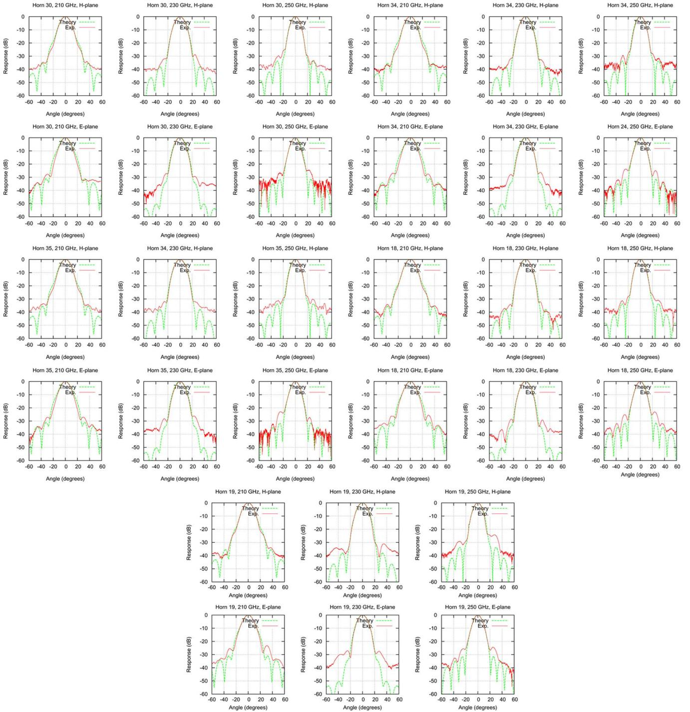
Fig. 15. Experimental and theoretical beam patterns for horns 30, 34, 35, 18, and 19. See Fig. 10 for their location within the array.
