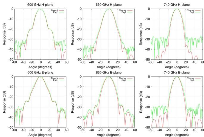
Fig. 17. Experimental and theoretical H and E plane beam patterns measured for the 700 GHz prototype horn, measured between 600 and 740 GHz. Top: H-plane, Bottom: E-plane.
