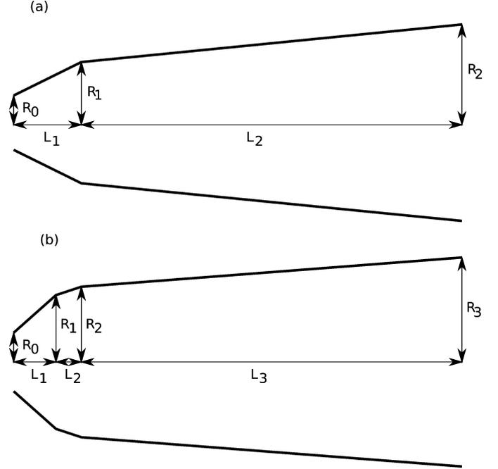
Fig. 1. A schematic diagram of (a) 2-section and (b) 3-section multiple flare-angle horns.
