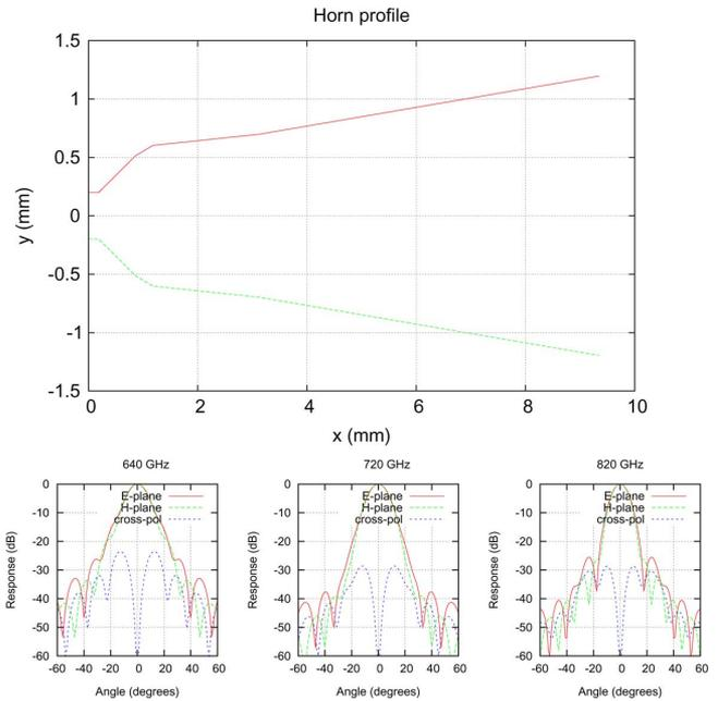
Fig. 19. Top: Profile of a new horn design designed with our GA software for extended bandwidth. Bottom: Simulated beam patterns for this horn design. The fractional bandwidth illustrated is 25%.
