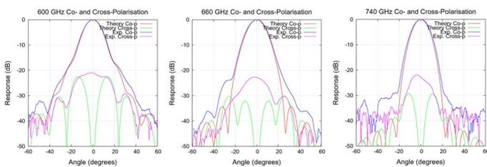
Fig. 18. Experimental and theoretical co-polar and cross-polar beam patterns measured for the 700 GHz prototype horn, measured between 600 and 740 GHz.
