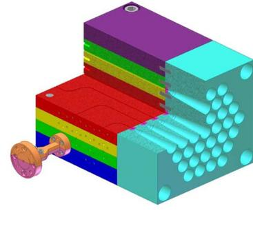
Fig. 9. The multi-plate split block enabling RF power to be delivered to each of the horns from a split block waveguide at the sides and rear.
