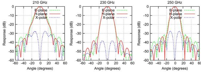
Fig. 2. Theoretical beam patterns (E plane, H-plane and cross-polarization) calculated using modal matching.
