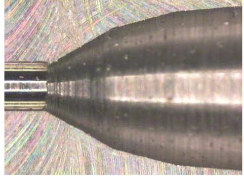
Fig. 5. The throat region of one half of the 230 GHz split drilled horn. For scale, the input waveguide on the left has a diameter of 1.24 mm.
