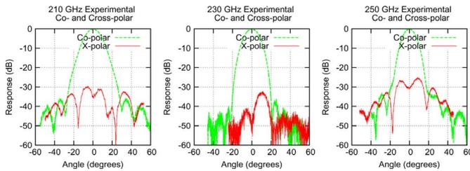
Fig. 7. Experimental co-polar and cross-polar beam patterns for the electroformed prototype horns.
