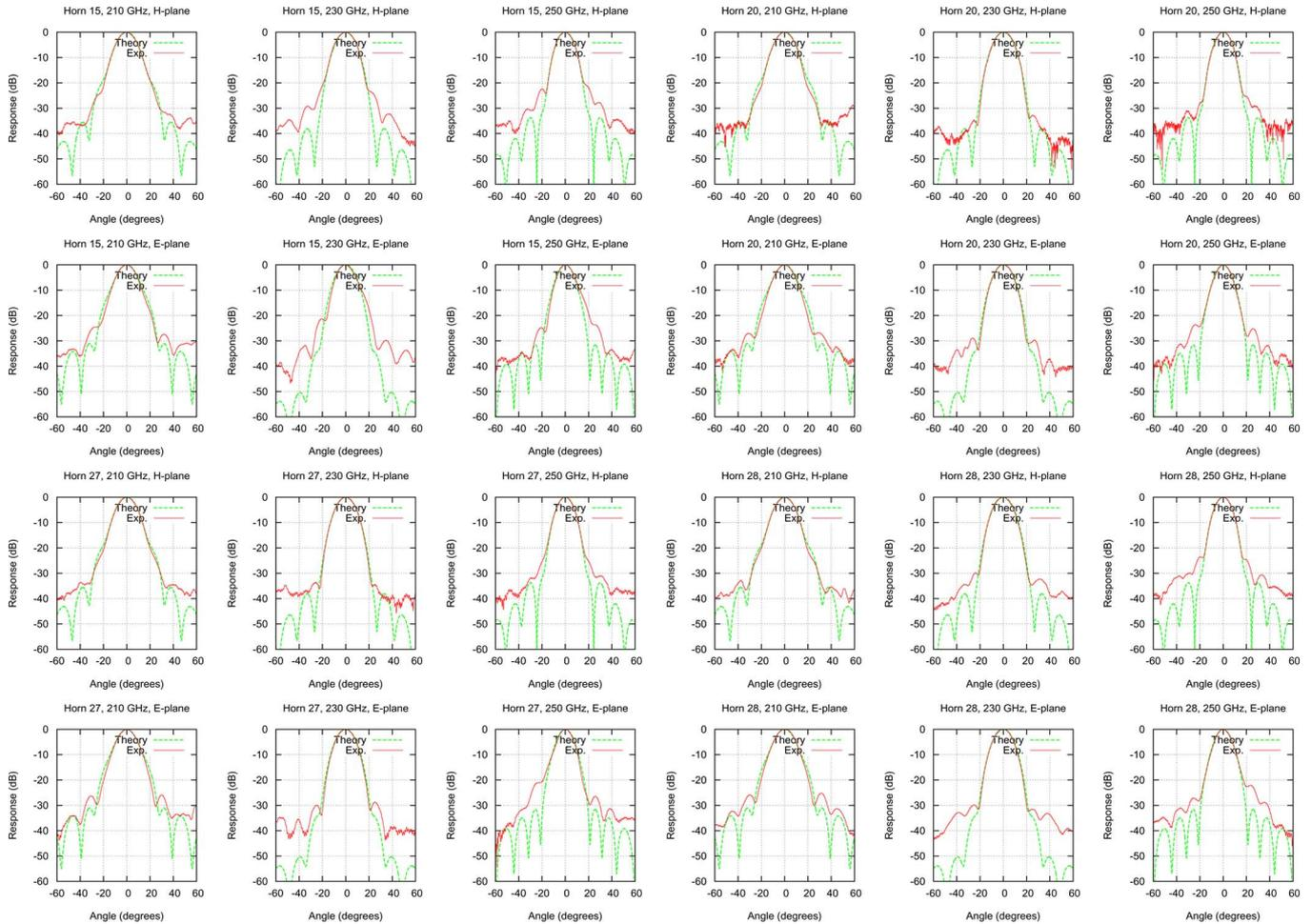
Fig. 13. Experimental and theoretical beam patterns for horns 15, 20, 27, and 28 from the 37-horn array. See Fig. 10 for their location within the array.
