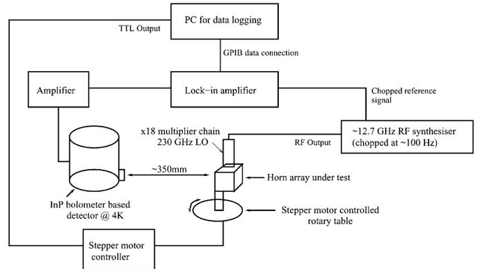
Fig. 11. A schematic diagram of the experimental test system used to test the 230 GHz 37-horn array.
