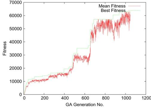
Fig. 3. A typical plot showing how the mean and peak fitness ( $\equiv 1/\delta^2$ ) increases with each successive GA generation.
