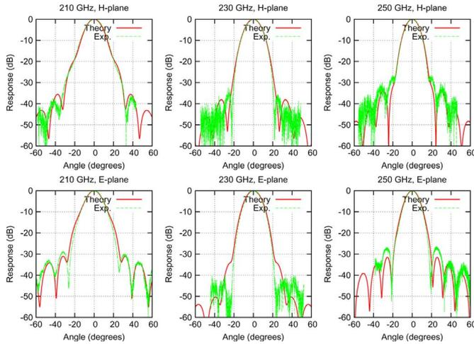
Fig. 6. A comparison of the theoretical beam patterns calculated using modal matching and the experimentally measured beam patterns for the electroformed prototype horns.
