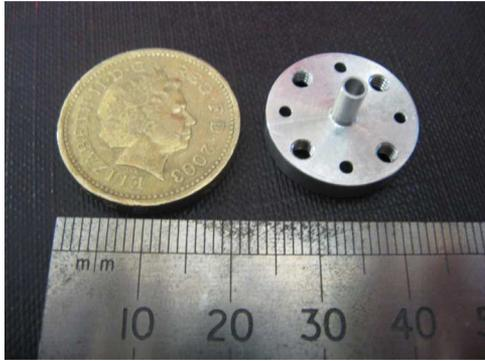
Fig. 16. The 700 GHz drilled horn prototype.
