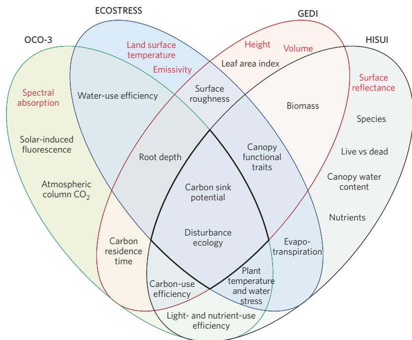
**Figure 1 |** Spatial and temporal synergy of observations and their applications. A pretzel diagram of observations (red text) from each instrument (coloured shapes) and the synergistic physical parameters that can be derived (black text) when observations are taken at synchronous and complementary spatial and temporal resolutions.
