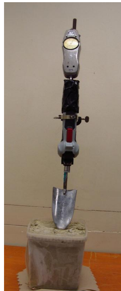
Figure 6: Autohammer testing setup. Top: force sensor; middle autohammer with trowel; bottom icy sand.
