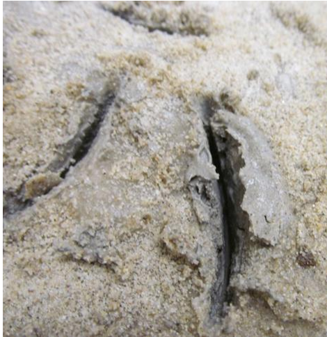
Figure 13: 2 cm penetration into icy soil with a force of 58 N using the autohammer. Notice the clay like behavior of the sand and water.
