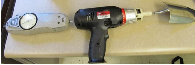
Figure 7: Percussive scoop prototype with force sensor (far left), hammer drill (center), and trowel (right).
