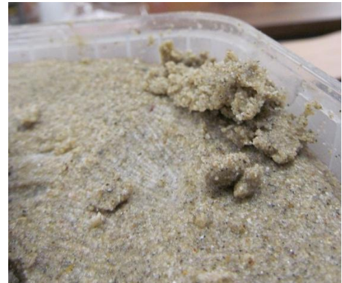
Figure 14: Lower angle scraping results using autohammer in icy soil.
