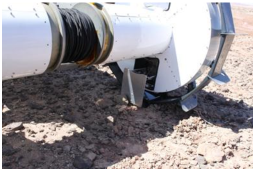
Figure 2: Axel instrument bay with deployed instrument panel
