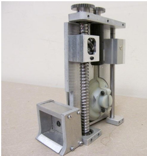
Figure 18: Actual design of percussive sampling system. Right: scoop; front right: ball screw with ball screw nut; white: part of autohammer percussive mechanism.
