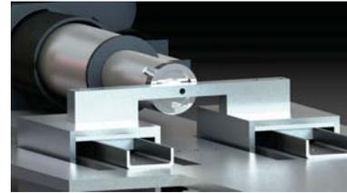
Fig. 5. Load cell mounted onto the actuator
