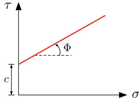
Fig. 1. Mohr-Coulomb failure criterion
