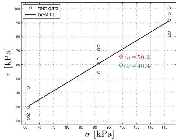
Fig. 9. Results of the in-situ simple shear test (blue circles) and corresponding best linear fit (black line)
