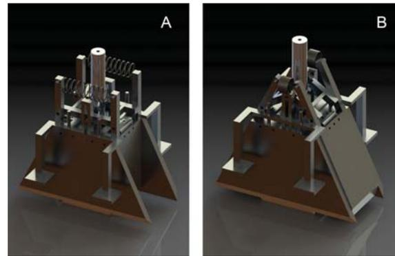
Fig. 6. A: Opening mechanism from isometric view (closed) B: Opening mechanism from isometric view (open)
