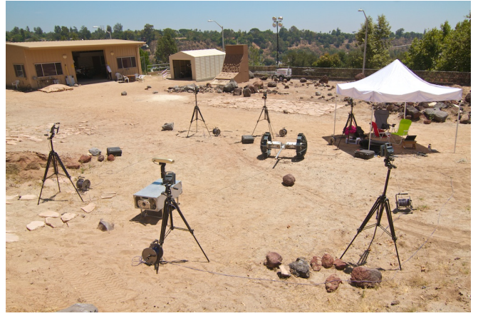
Fig. 8: Autonomous docking experiments with the VICON ground truth system in the JPL Mars Yard.
