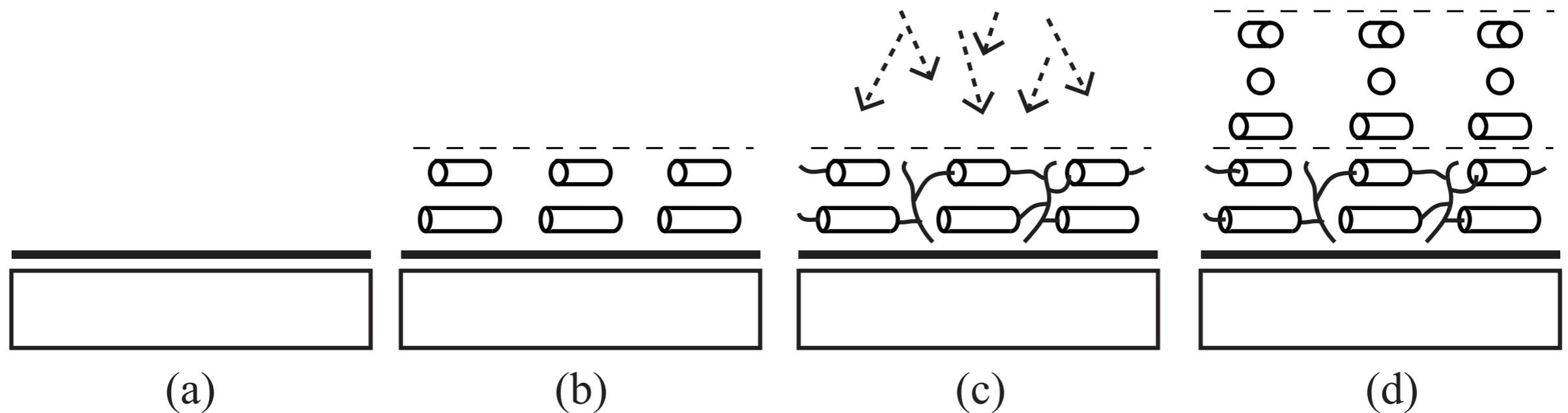
Fig. 8. The MTR fabrication procedure resulting in a monolithic broadband element, on a single substrate and alignment layer: (a) alignment layer processing; (b) LCP coating ( $m = 1$ ); (c) LCP photo-polymerization; and (d) repeat LCP coating and curing for ( $m \geq 2$ ).
