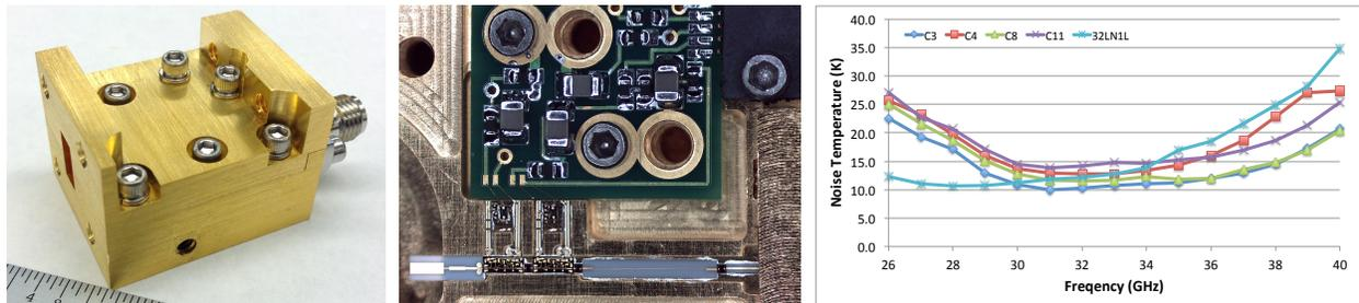
*Figure 2:* (Left) Exterior of a COMAP amplifier module. (Center) Interior of the amplifier module, showing RF and DC-bias components. (Right) Noise measured on four such modules, showing noise temperatures of 10-15 K in the main COMAP band of 30-34 GHz. Also shown is the noise temperature of a single 32LN1L amplifier, which has been optimized for the new COMAP band of 26-34 GHz.
