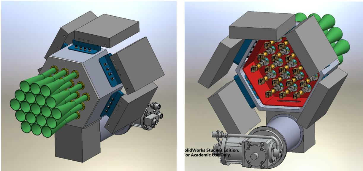
*Figure 5* Renderings of preliminary design for COMAP receiver cryostat. The 19 warm feeds of the array can be seen on the left. Arrayed around the outside are the 5 first-stage mixer chassis. The cold head is offset to allow easy access to the amplifier modules from behind (right).
