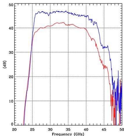
*Figure 3:* Measured room temperature (red) and cryogenic (blue) gain of a typical amplifier module.
