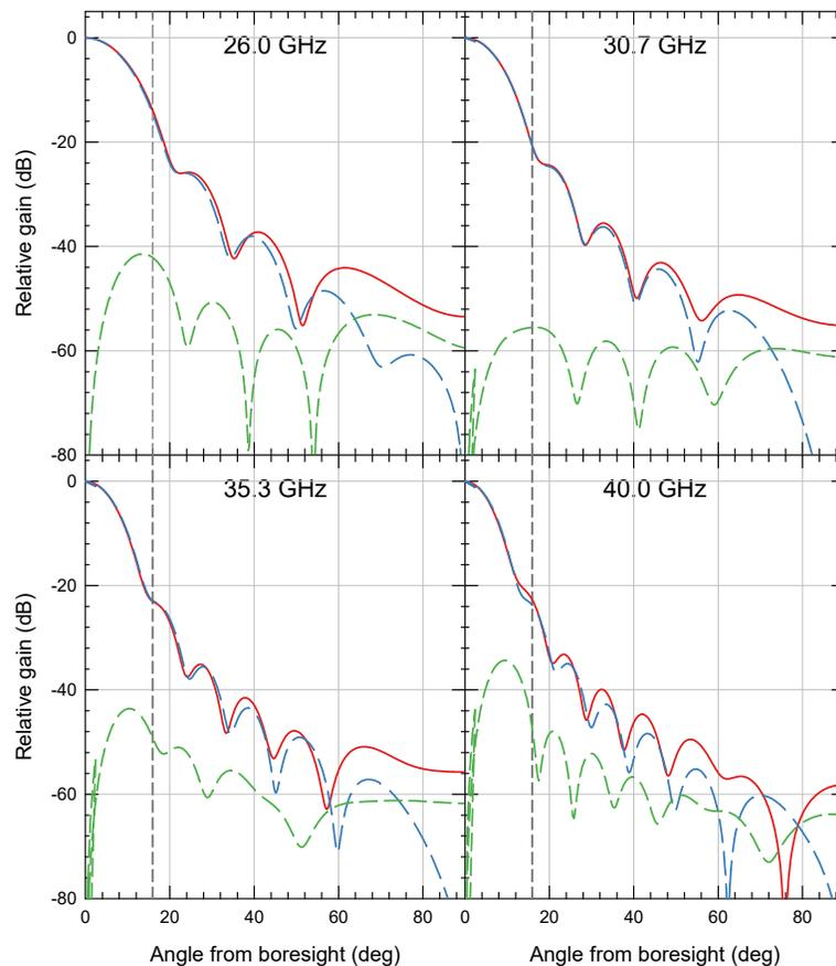
*Figure 4:* Beam simulations for the 10m optical design (blue: E-plane, red: H-plane, green: polarization in 45-degree plane) at four frequencies in the 26-40 GHz range.
