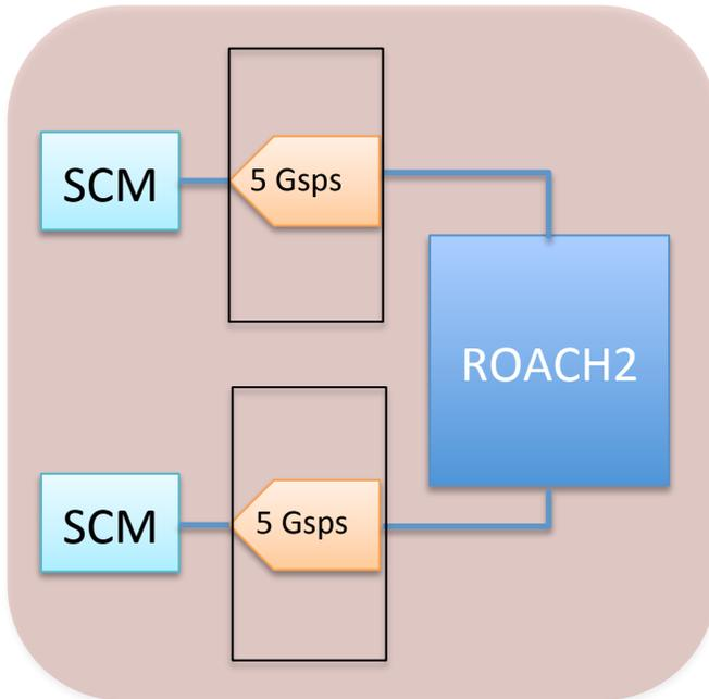
*Figure 6:* Digital backend design based on CASPER hardware. A signal conditioning module (SCM) conditions the signals from the receiver for input to a 5 Gbps digitizer. Two such digitizers are controlled by a single 'ROACH2' FPGA board. This backed unit will process 4 GHz from a single polarization – the full digital backend will require 38 such units to process 8 GHz from each of 19 pixels.
