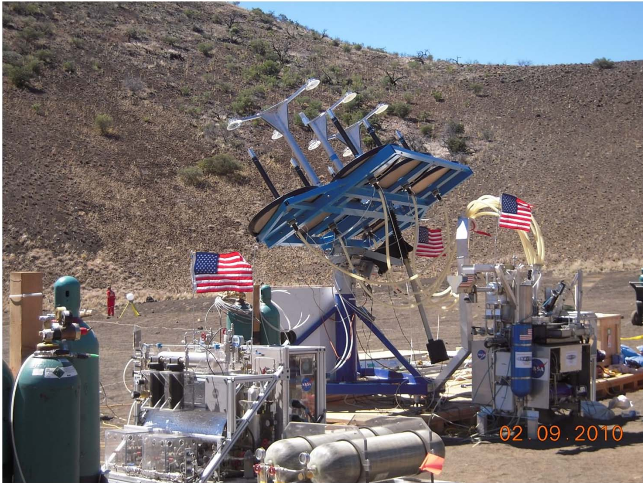
PSI Solar Concentrator (middle), ORBITEC CT Reactor (right) and NASA/JSC Water Electrolyzer (left) operated remotely from Houston, TX
