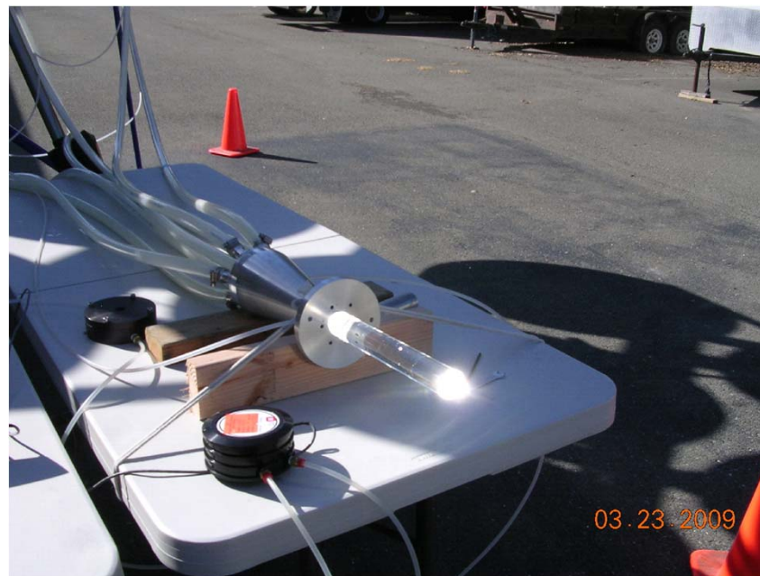
The quartz rod emitting solar radiation
