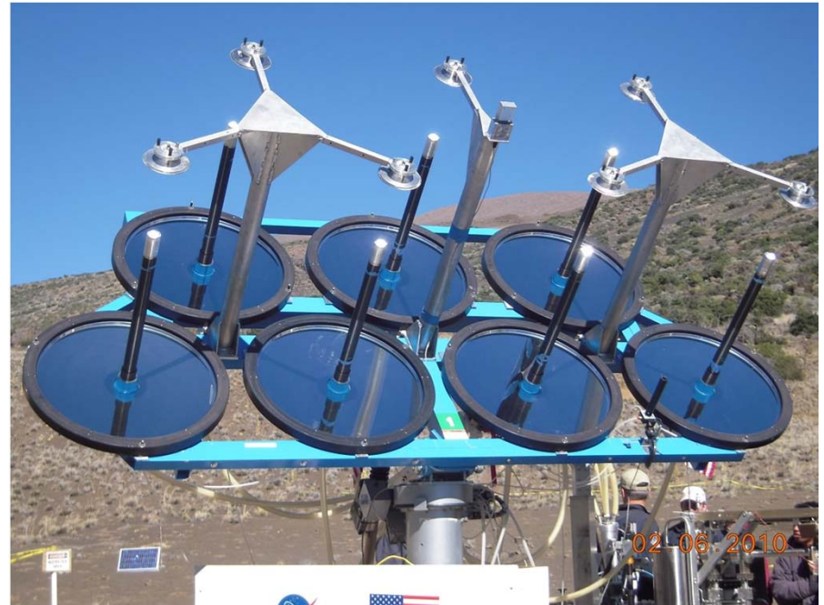
Seven Primary Concentrators Cleared of Dust Deposit • 10% Power Increase by Cleaning
