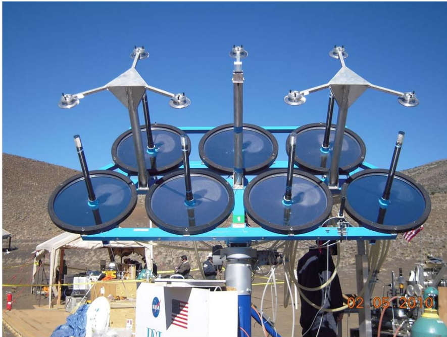
Dust Deposit on the Primary Concentrators
