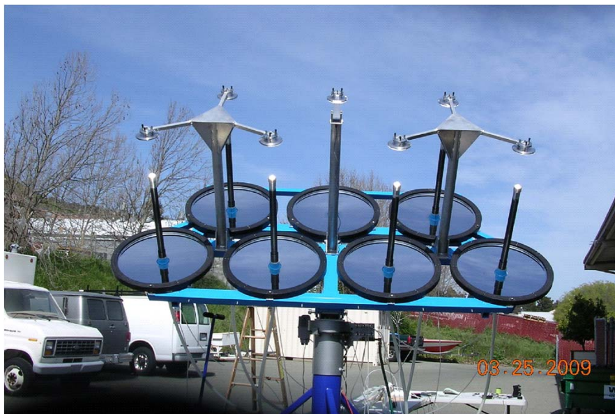
Seven concentrators mounted on the tracking array
