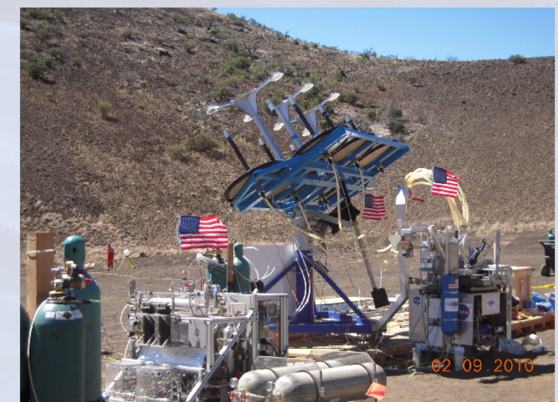
PSI Solar Concentrator (middle), ORBITEC CT Reactor (right) and NASA/JSC Water Electrolyzer (left) operated remotely from Houston, TX
