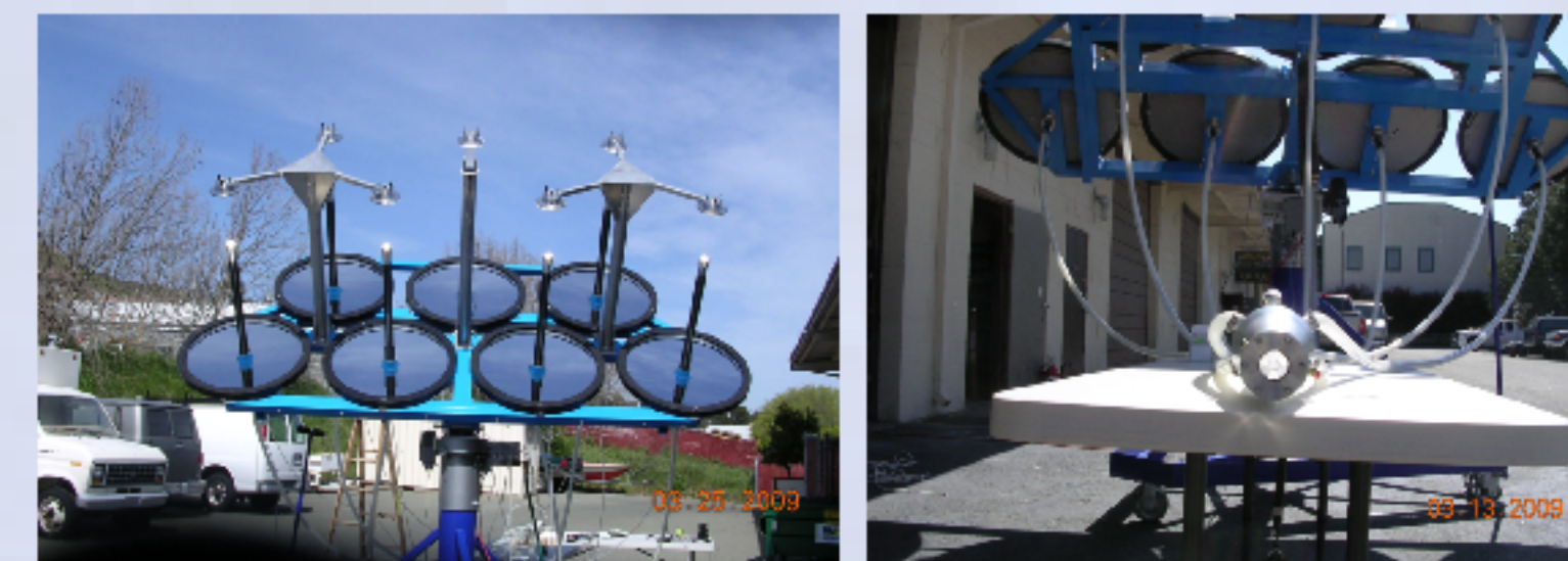
Seven concentrators mounted on the tracking array
