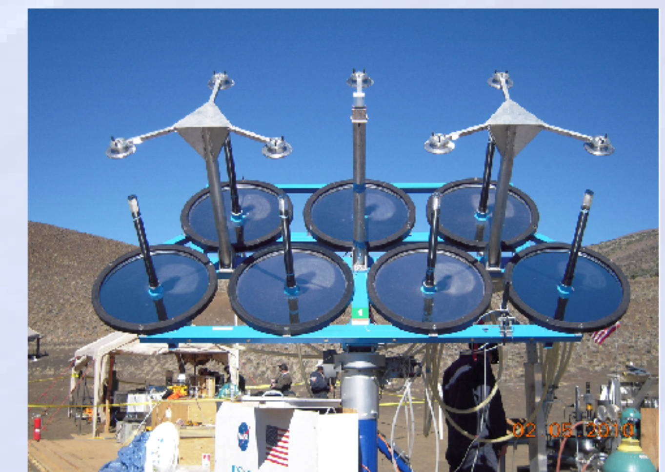
Dust Deposit on the Primary Concentrators
