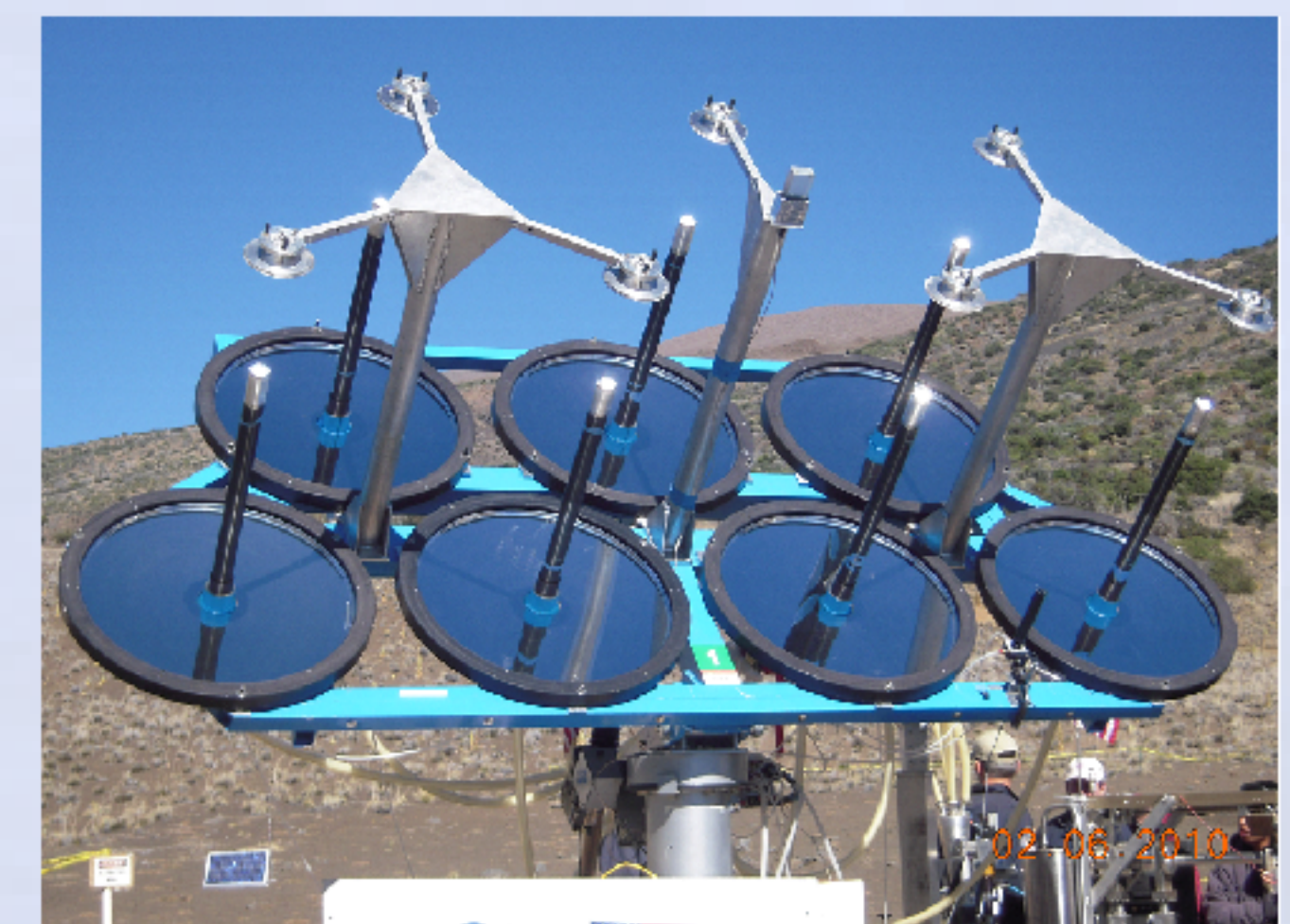
Seven Primary Concentrators Cleared of Dust Deposit • 10% Power Increase by Cleaning
