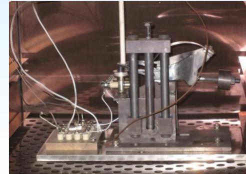
Wireless seismometer and circuit in an oven at 500°C
