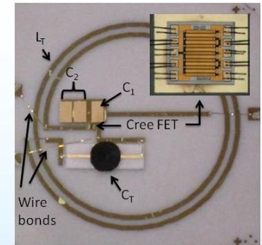
Wireless Pressure Sensing Circuit
