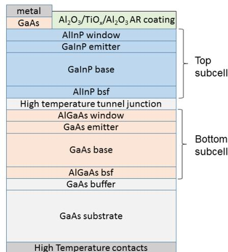
Simplified cross-section schematic of a GaInP/GaAs 2J solar cell designed for high temperature operation.
