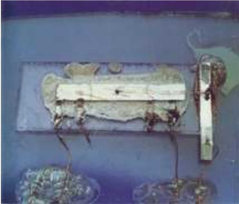
Kilby's first integrated circuit
