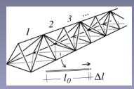
GMTI Space-Based Radar Antenna: Triagonal bay antenna support structure
