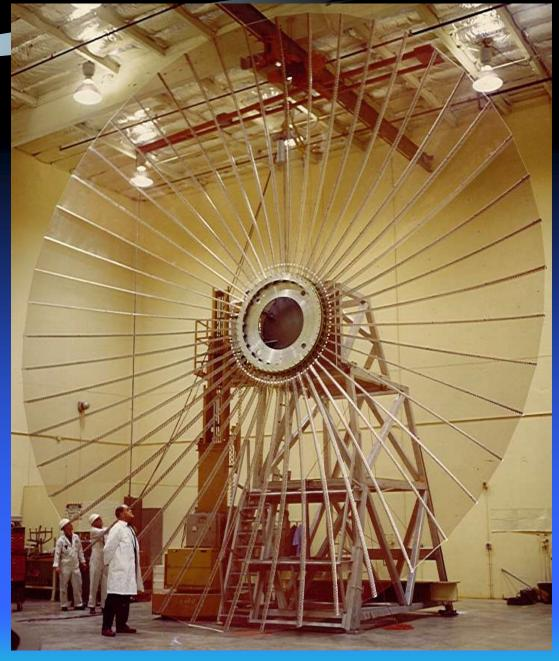
Lockheed LSST: Wrap-Rib Antenna (sector of 55m dia.)
