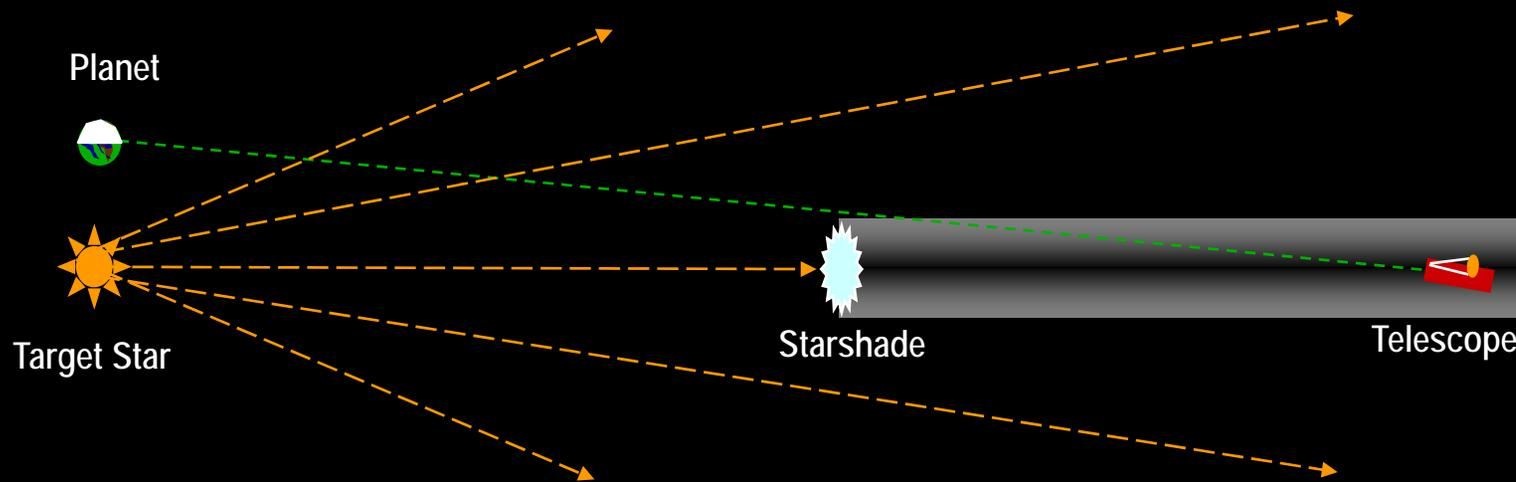
**Characterizing Exoplanets:** Via the use of an external occulter, one can suppress the light of the central star, enabling the detection of any orbiting exoplanets. Detecting and characterizing these, however, becomes progressively easier with increasing telescope aperture.
