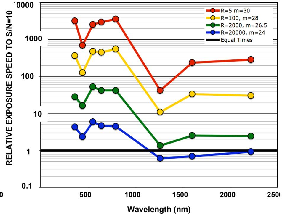
8-m ST faster than 30-m on ground for all imaging and for most R=100 low-res spectroscopy. 8-m also faster for med-resolution spectroscopy in optical band.
