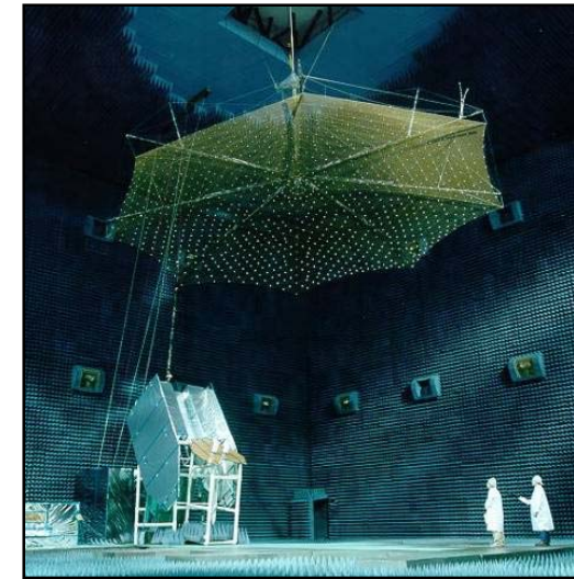
ACeS Folding Rib in RF Test
