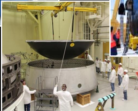
Diaphragm installed and tested on MSA in support of EFT-1
