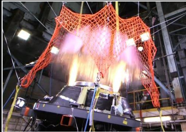
Forward Bay Cover Jettison Test Denver, CO
