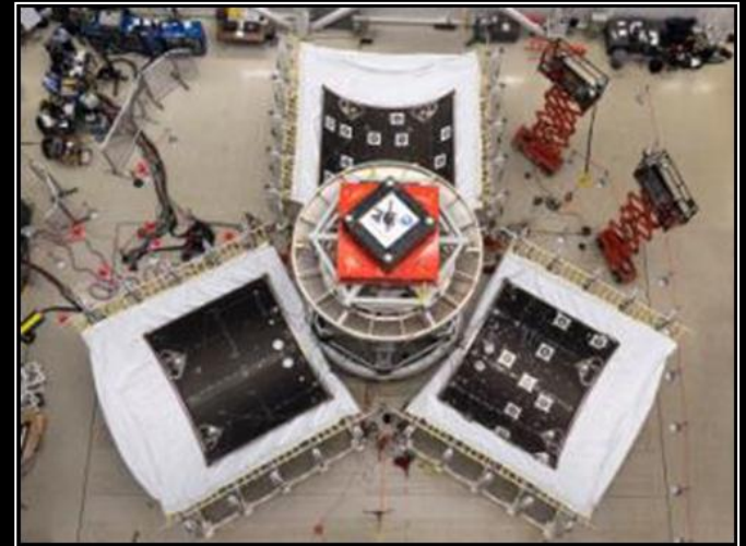
Fairing separation test at Lockheed Martin, Sunnyvale, CA
