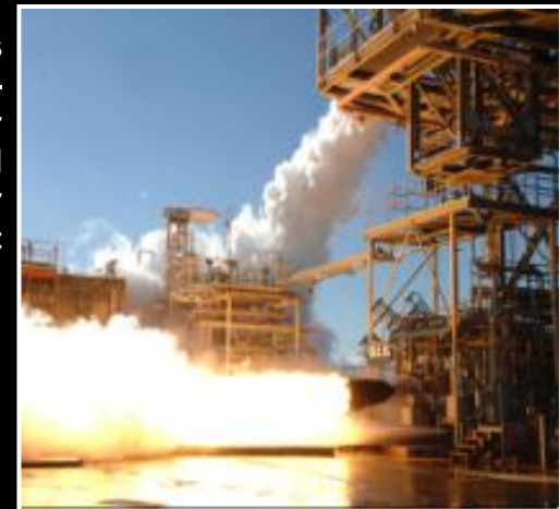
F-1B gas generator – tech demo for advanced booster concept
