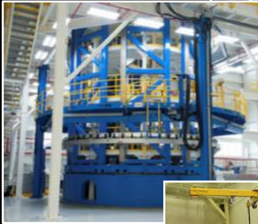
Vertical weld tool complete at Michoud Assembly Facility
