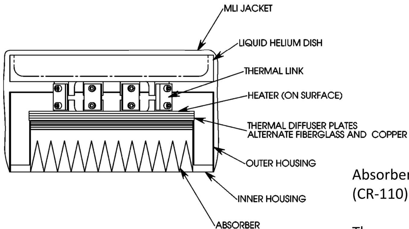
Absorber is iron loaded epoxy
