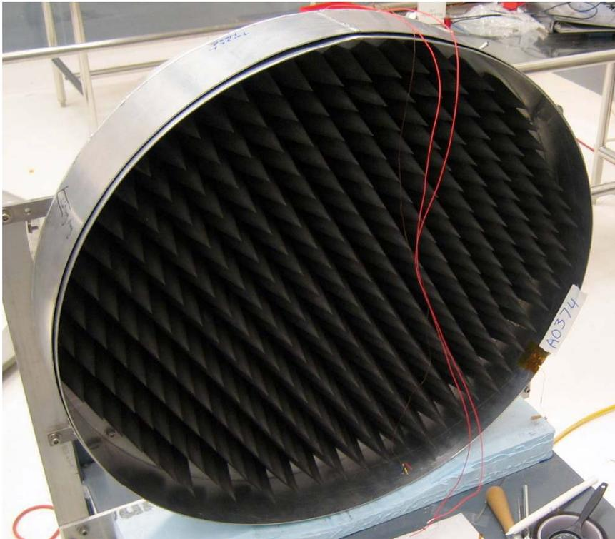
Absorber cones cast onto aluminum core
