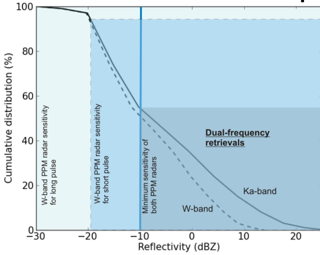
Figure 3.1: Cumulative distribution of Ka and W radar reflectivity of snow climatology in Finland. The measurements are converted from C-band weather radar observations (Leinonen et al., 2010). The blue line shows the minimum sensitivity requirement for PPM dual-frequency radars.
