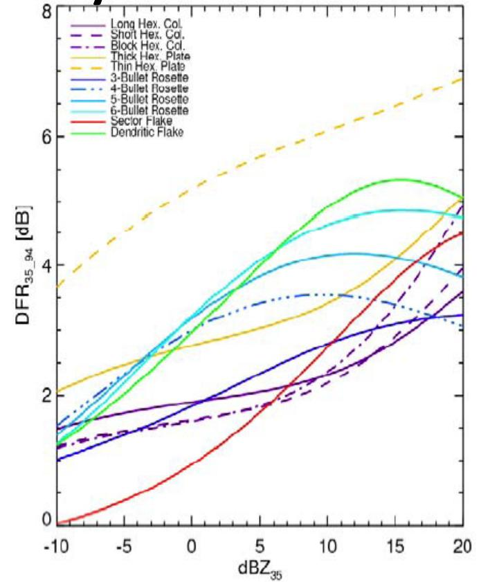
Figure 3.4: Simulated 35/94 GHz dual-frequency ratios as a function of 35 GHz reflectivity for various ice particle habits (Liu, 2008) using ice PSD parameterization (Field, et al., 2005). (Figure from Kulie and Bennartz, 2009)
