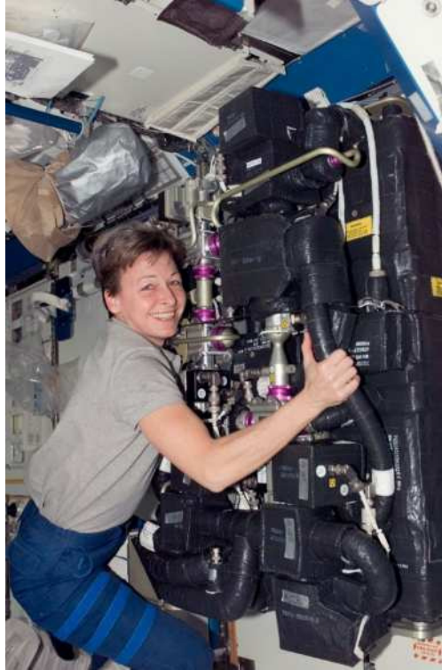
Figure 7: Astronaut Peggy Whitson on ISS Expedition 16 Performing In-flight Maintenance on the Carbon Dioxide Removal Assembly
