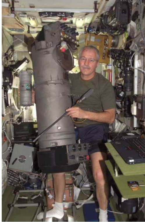
Figure 8: Astronaut John Phillips on ISS Expedition 11 Performing Repairs on the Russian ELEKTRON O 2 Generation System
