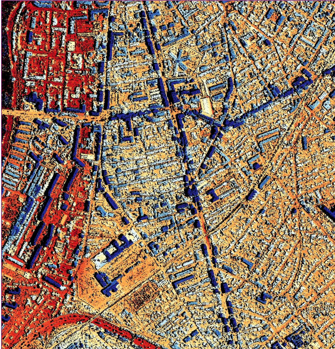
DSM generated with a stereoscopic couple.
