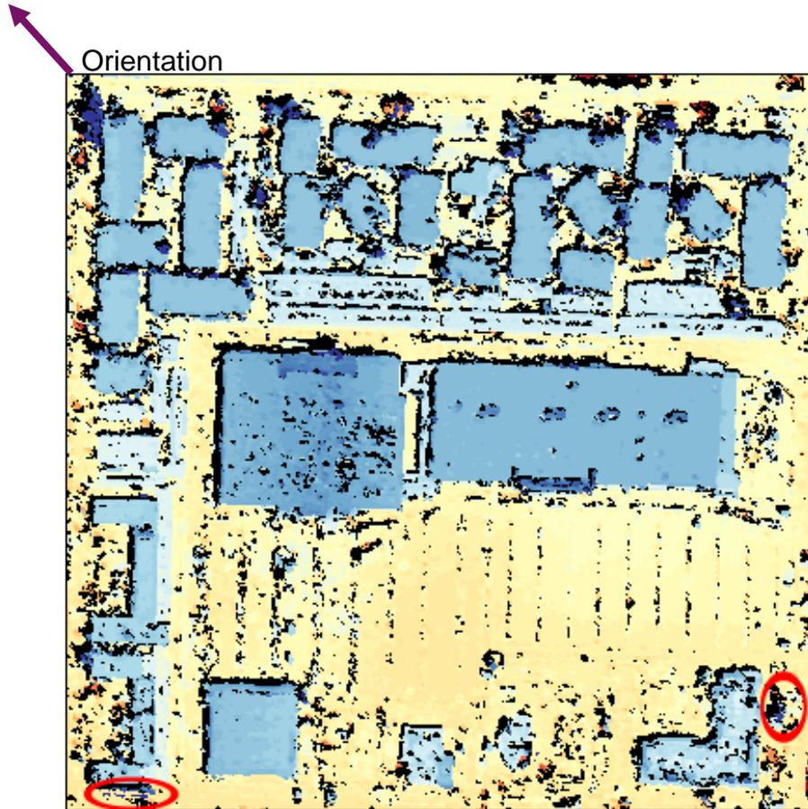
Elevation image from the image 1 resampled onto a geographic grid
