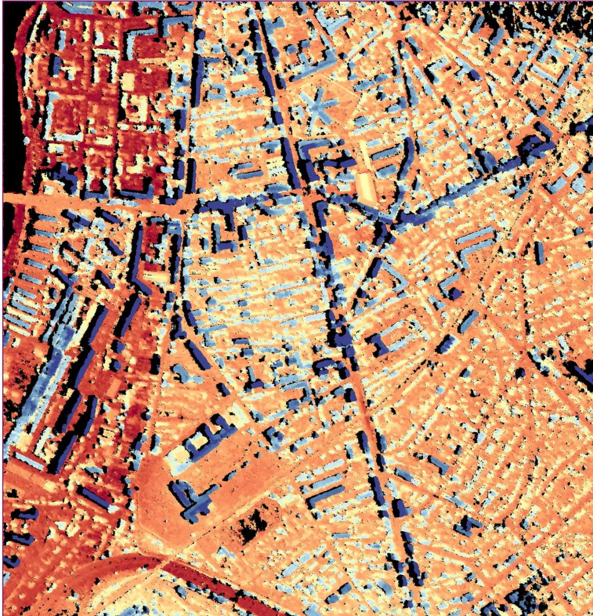
DSM generated with a tri- stereoscopic couple.
