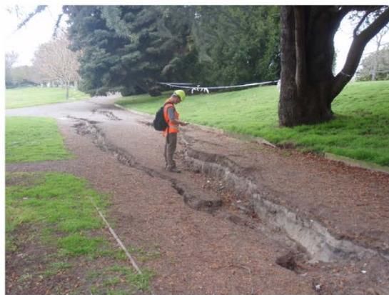
(b) Tracing crack with GPS
