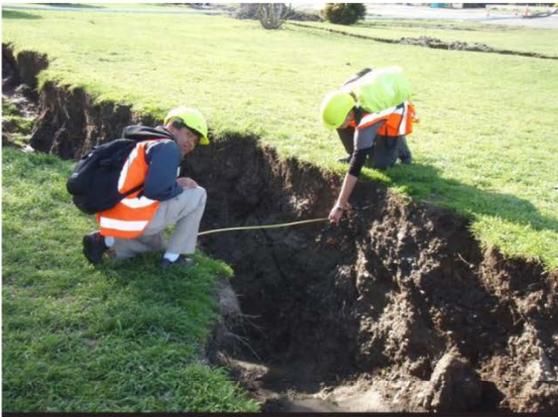
(a) Measuring crack width
