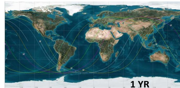
Immediately after launch, all satellites (blue lines) are in the same orbit plane. Due to slightly different precession rates (due mostly to different satellite altitudes), the satellite orbits spread over time such that within a year they are spread equally over the globe.
